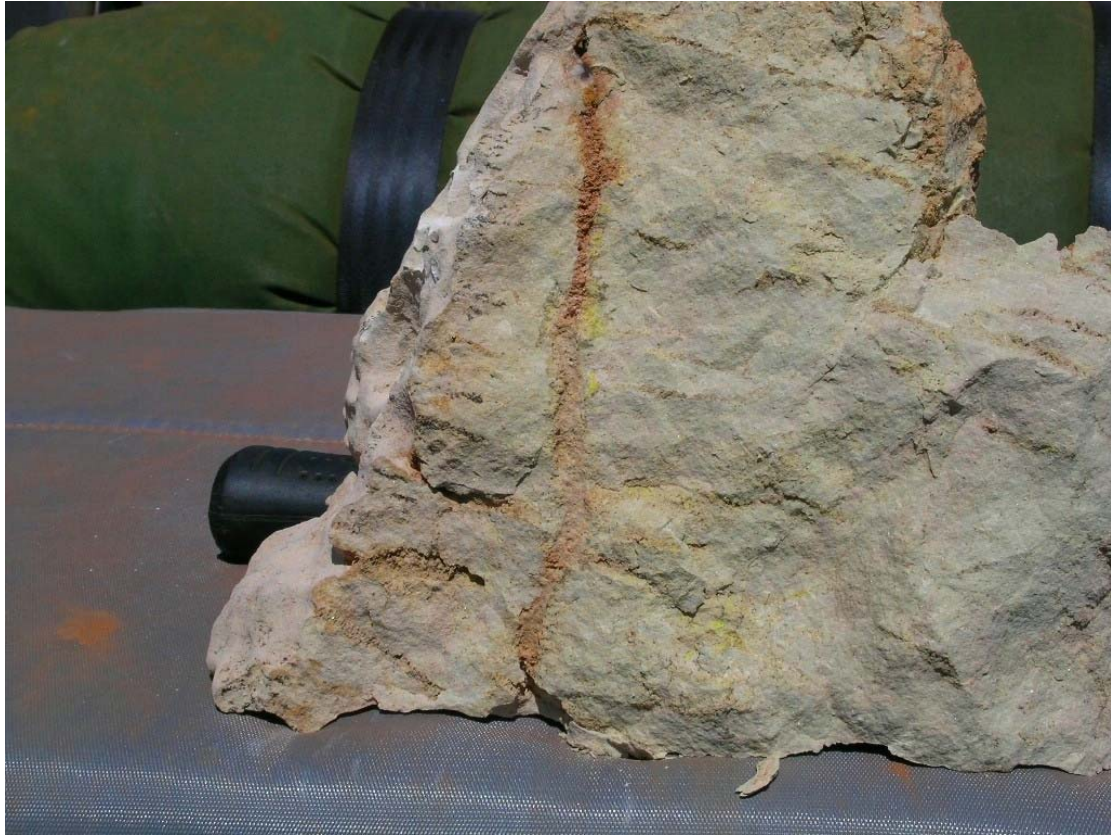
Figure 2: Visible Carnotite in sandy limestone from Newera's Ben Hur prospect within E09/1194 of Newera's Jailor Bore project .
